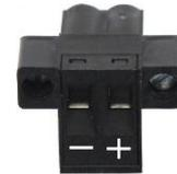
The power connector (Molex 2 pin female) is supplied fitted to the radio. Wire your power source to the power connector (- / +) and plug the connector into the radio. The connector screws should be fastened to secure the connector.
